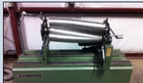
All Scrolls are Remanufactured and Precision Balanced Prior to Installation
